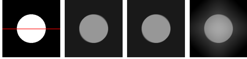
(a) Symmetric data (b) TV solution, \alpha = 10 (c) TGV solution, \alpha = 10, \beta = 10^6 (d) TGV solution, \alpha = 10, \beta = 200
