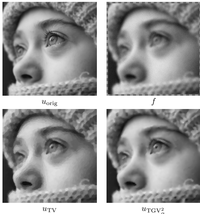
Fig. 2. Deconvolution example. The original image u_{\text{orig}} [7] has been blurred and contaminated by noise resulting in f , u_{\text{TV}} and u_{\text{TGV}_\alpha^2} are the regularized solutions recovered from f .
