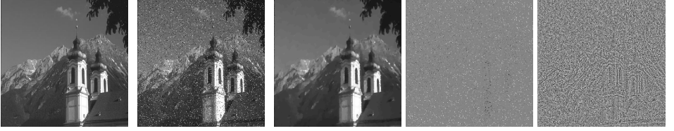
Figure 15: Optimal impulse-Gaussian denoising. From left to right: Original image, noisy image corrupted by impulse noise and Gaussian noise with mean zero and variance 0.005, denoised image, impulse noise residuum and Gaussian noise residuum. Optimal parameters: \lambda_1^* = 734.25 and \lambda_2^* = 3401.2 .
